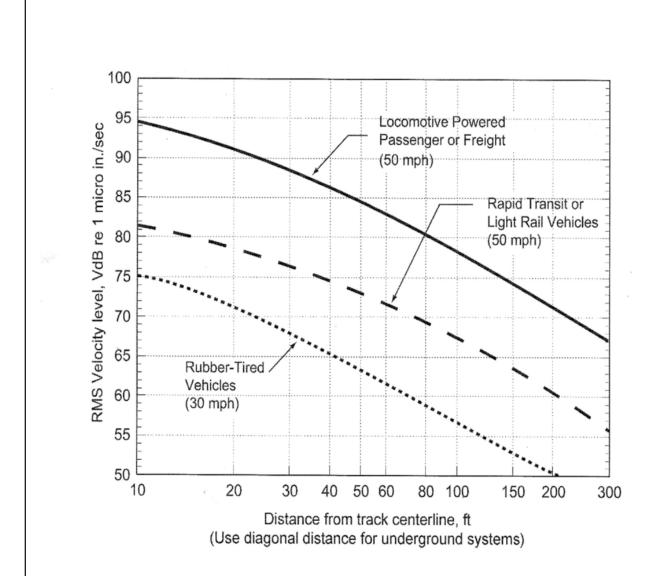
\*The above curves represent the upper range of measurement data and it is rare that groundborne vibration will exceed these curves.
