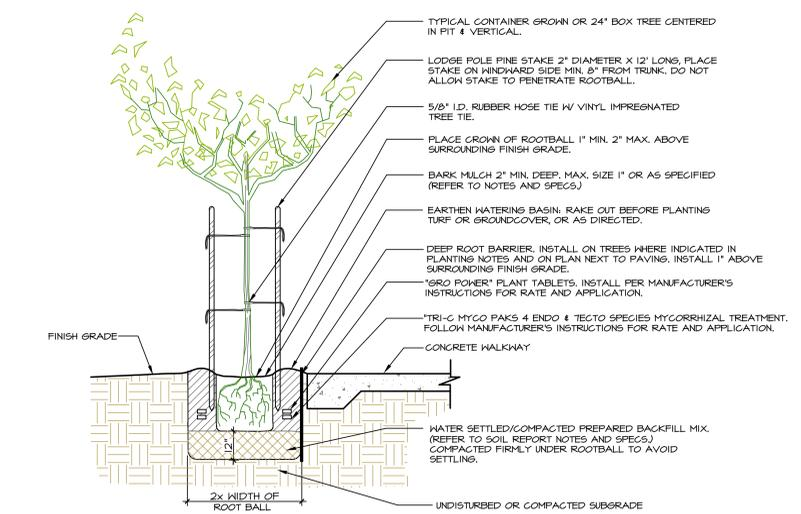
**A TREE STAKING W/ DEEP ROOT BARRIER DETAIL**
