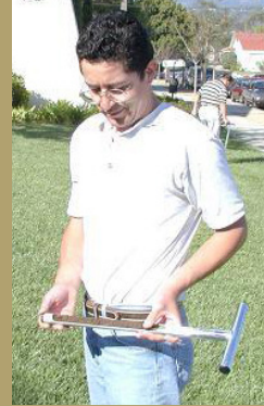
Soil type and moisture can be assessed with a soil probe.
