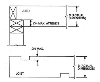
NOTE: Notching not permitted in middle of 1/3 of span
