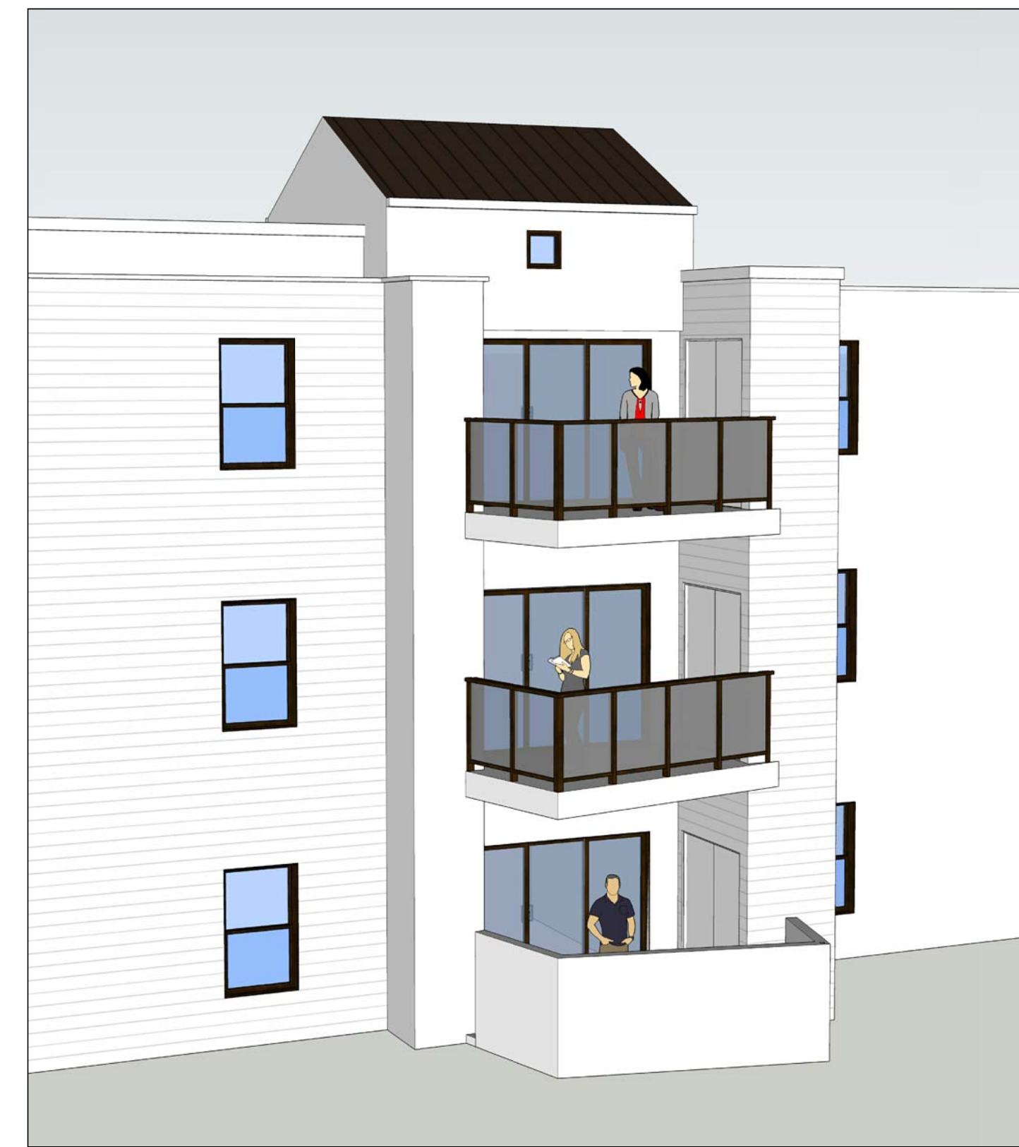
STANDARD RAILING (NO SOUND BARRIER)
