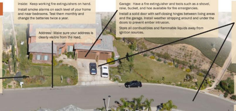
Driveways and Access Roads: Driveways should be designed to allow fire and emergency vehicles and equipment to reach your house.
